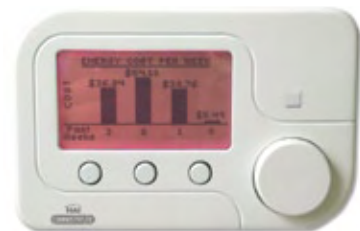
This graph allows you to monitor your Energy Cost, broken down by a specified time determined by your energy company.*
