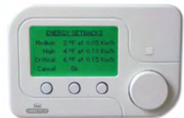
Displays Energy Setbacks for medium, high, and critical energy rates. These automatic temperature setbacks allow you to save money on energy bills if rates were to change.*
